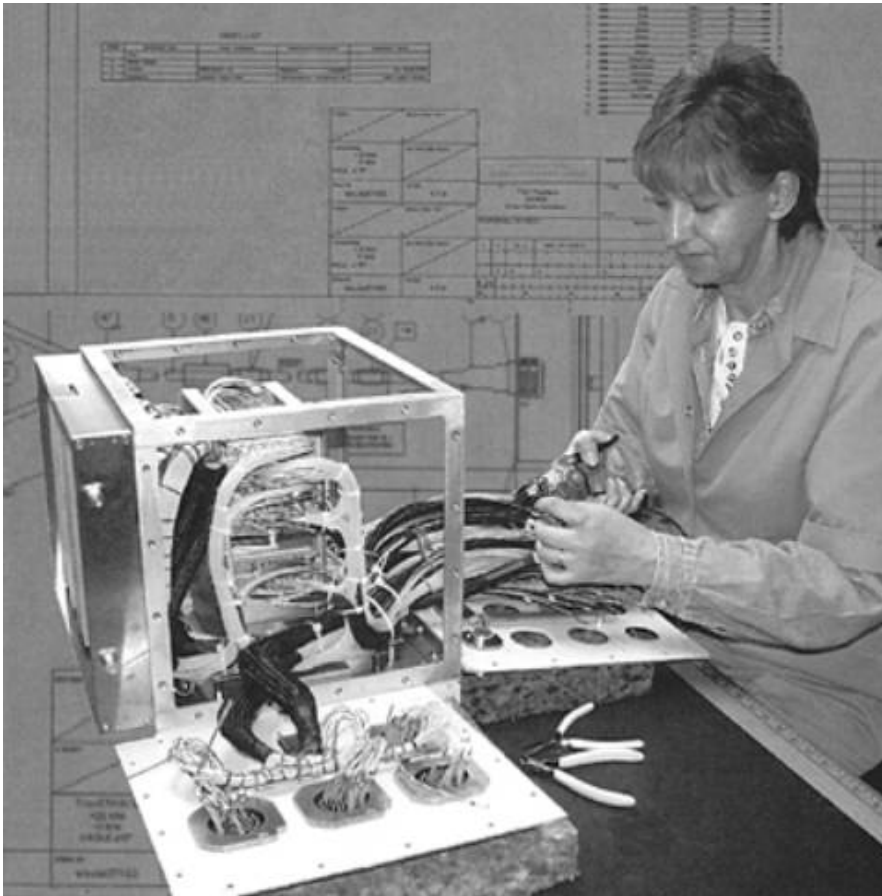
Photograph shows an operative wiring up an interface adaptor for the Merlin avionics test set (MATS), which Rockford manufactured for Serco Test Systems.
