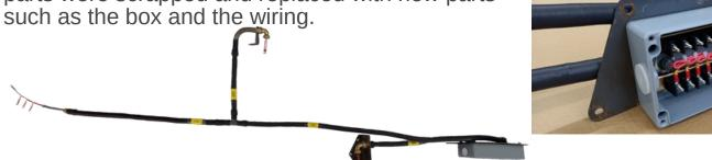
We then re-assembled the system using the agreed works orders and manufacturing instructions. The assembly was tested part by part in an agreed sequence, with testing of appropriate sub systems such as the wiring loom/junction box as part of process. Final testing included visual, physical and electrical tests.
